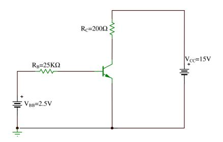
Given that for this transistor,  $V_{\rm BE} = 0.7V$  and  $\beta_{\rm DC} = 250$ , determine for the circuit;
