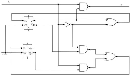
The circuit has one input A, one output Y and two state variables  $Q_1$  and  $Q_2$
