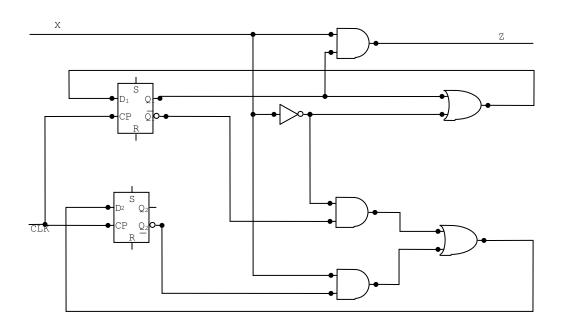
The circuit has one input X, one output Z and two state variables  $Q_1$  and  $Q_2$
