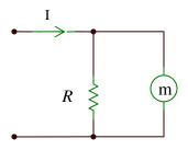
If the meter has internal resistance  $(R_m)$ ;
