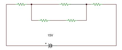
Assuming that each resistor is  $5\Omega$ , Calculate;
