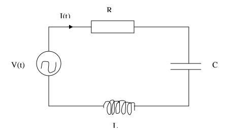
a) Express the voltage equation of the circuit as a second order differential equation in q.
