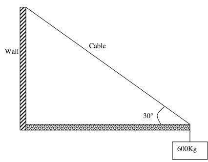
Assuming that the beam's mass is so small compared to that of the load and thus can be ignored, calculate;
