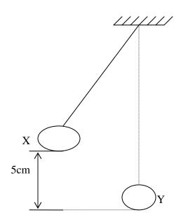
The length of the string is 80*cm* and the bob is momentarily at rest at point X, calculate the velocity of the bob when crossing point Y. (3marks)
