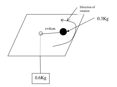
The 0.3Kg mass rotates in a horizontal circle of radius 4cm. Calculate the angular velocity ( $\sigma$ ) of the 0.3Kg mass for the system to be in equilibrium (4marks)
