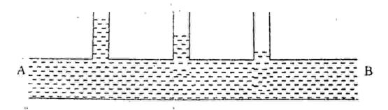
(i) Indicate the direction of the flow in the main pipe.
