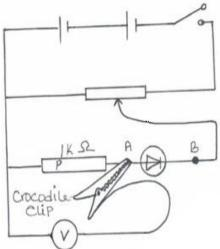
Starting with the crocodile clip connected to terminal A, adjust the potentiometer until the (xii) voltmeter reads 1.20 volts. Now move the crocodile clip to terminal B. Record the new voltmeter reading.
