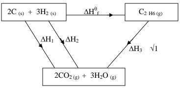
$$\begin{array}{ll} \Delta H^{\theta}_{\ f}(C_2H_6) &= 2\Delta H_1 \ + \ 3\Delta H_2 \ - \ \Delta H_3 \\ &= 2 \ (-394) \ + \ 3(-286) \ - \ (-1560) \ \ \sqrt{1} \\ &= -788 - 858 \ + \ 1560 \\ &= -86 \ kJmol^{-1} \ \ \ \sqrt{1} \end{array}$$
