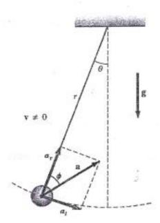
When the string makes an angle  $\theta$ =20° with the vertical, the ball has a speed of 1.5 m/s.
