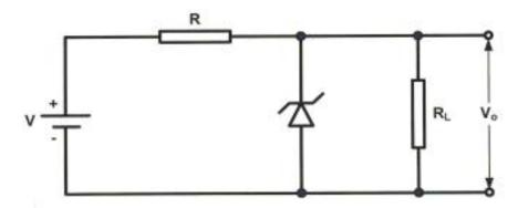
Assume that the supply voltage,  $v_s$  is 9 volts, and that the zener voltage,  $V_z = V_o = 6 \text{ V}$ If the maximum zener current that can safely flow is 20 mA.
