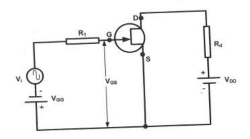
The operating parameters are:  $I_{DSS} = 10 \text{ mA}$ ,  $V_p \{ = V_{GS} \text{ (off)} \} = -3 \text{ V}$ ,  $V_{DD} = 25 \text{ V}$ ,  $I_D = 5 \text{ mA}$ , and VDS = 5 V, determine:
