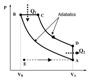
Fig. 3. P-V diagram for an ideal diesel engine
