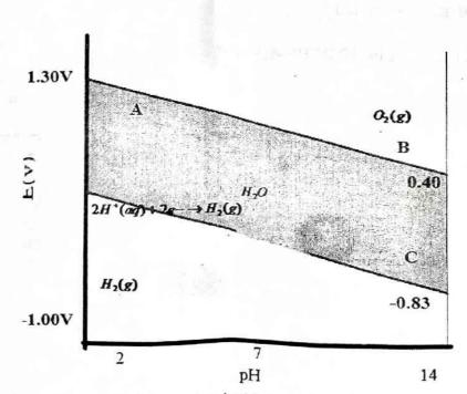
The graph above shows the electrochemical behaviour of water at various pH values
