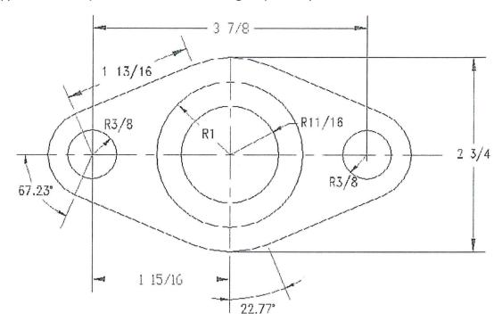
(g)Describe the steps Using Ortho and Direct Distance Entry of drawing the following shape(without dimensions) using the Plinecommand with width = 0.1.(6 MARKS)
