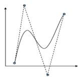
Approximating spline control points merely influence shape (Hermite Curves, B-spline)
