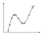
Interpolating spline curve passes through the control points knots (Cardinal spline, Catmull-Rom spline)
